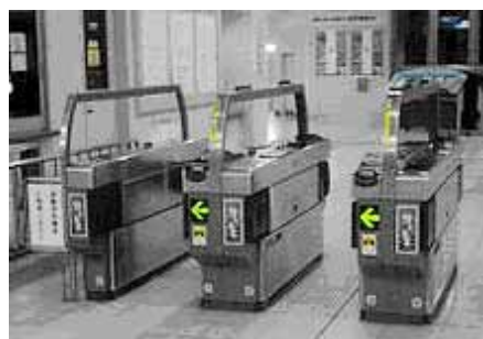
Automated ticket gate
